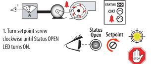
2. Slowly turn the screw counter-clockwise until the Status CLOSED LED just turns ON.
