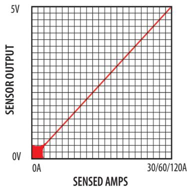
\*Factory calibrated ranges selected with the amperage range switch
