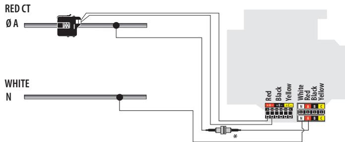
\* External fuse provided by installer (optional, per NEC and local regulations).
