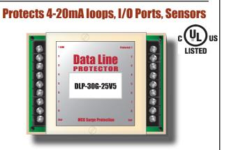
The DLP-10G/20G/30G Series are triple-stage hybrid protectors that combine brute force primary protection with high speed silicon avalanche diode stages for rigorous transient clamping.
