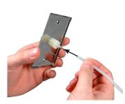
1. Connect tubing between the fitting on the PX sensor and the fitting on the back of the AA56.
