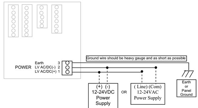
Figure 3: Power Supply Wiring
