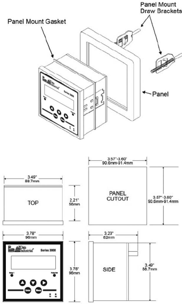
Figure 1: Panel Mounting Dimensions
