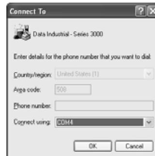
5. Configure this Port with 38400 baud, 8 data bits, 1 stop bit, no parity, and no flow control.
