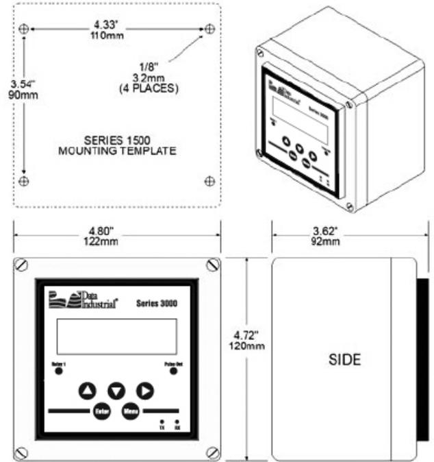
Figure 2: Wall Mounting Dimensions
