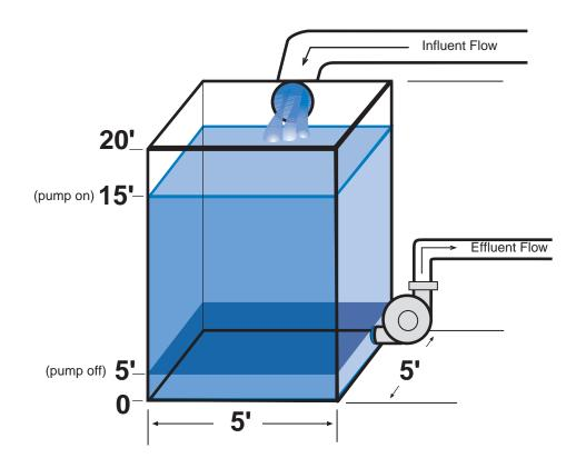
Well volume =  $(5 \times 5) \times (15 - 5) = 250$  cubic feet 1 cubic foot = 7.48052 gallons Well volume = 250 cubic feet x 7.48052 gallons/cubic foot = 1870 gallons
